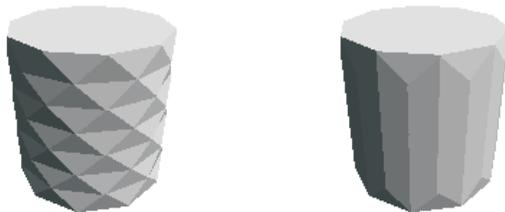
Figure 2: Two examples of triangulation. Left: Delaunay triangulation; Right: Tightest triangulation. Adapted from [1]
